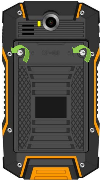
**!** Turn the screw lock to the left on the battery cover till it loosens
