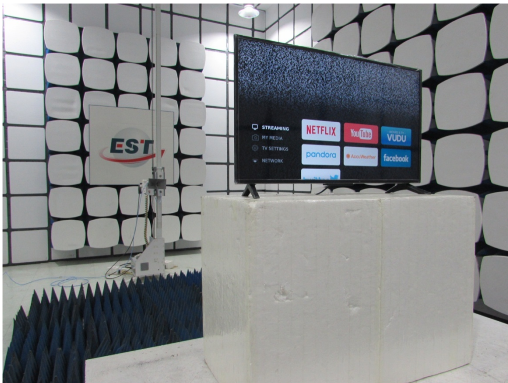
Radiated Test (Above 1000 MHz)
