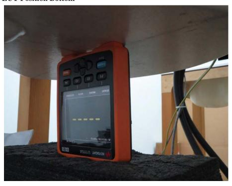
The EUT (the bottom of EUT site) to the ELI4 phantom distance is 0 mm.
