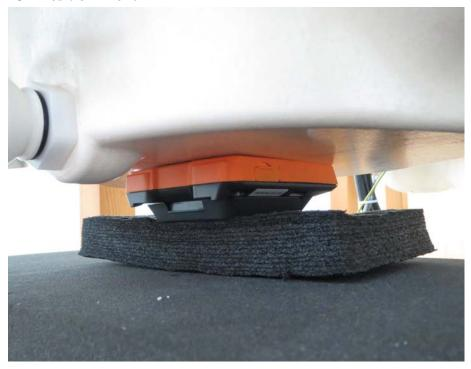
The EUT (the bottom of EUT site) to the ELI4 phantom distance is 0 mm.
