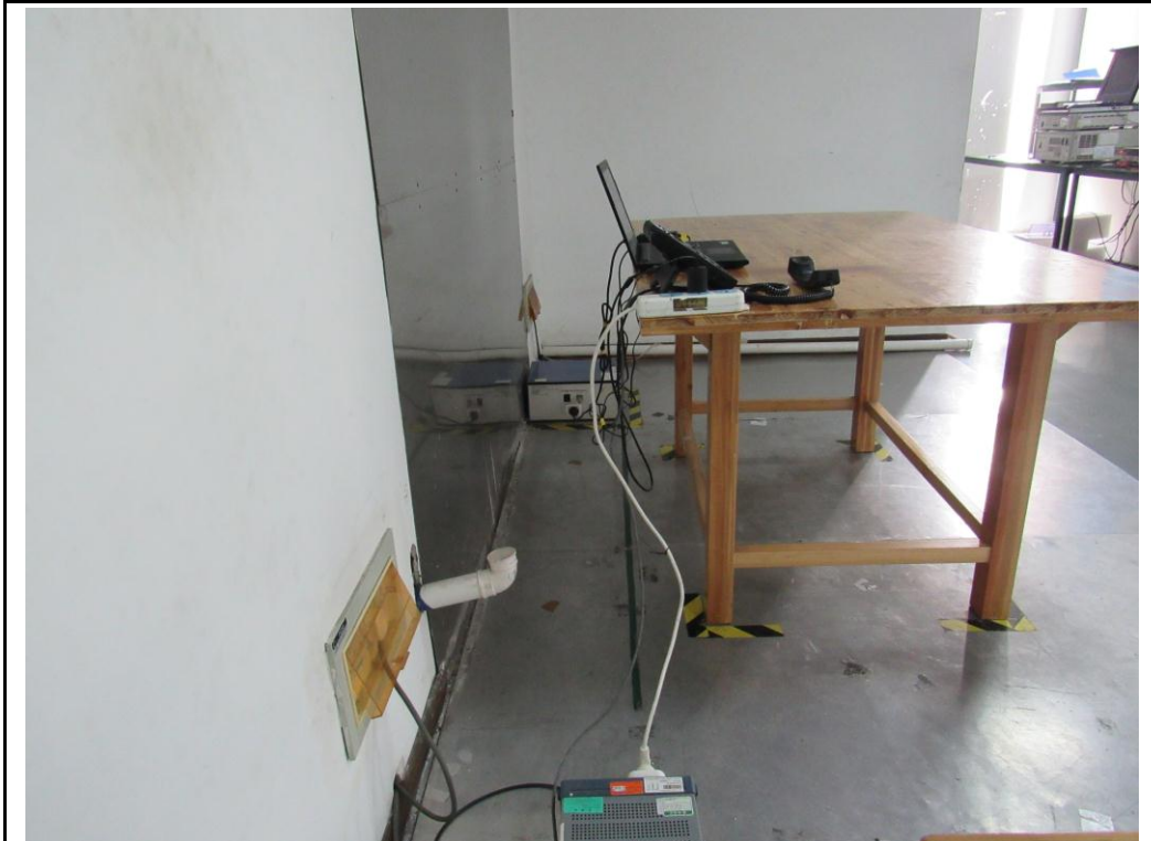
Conducted Emissions Test Setup Side View – Adapter Power Supply
