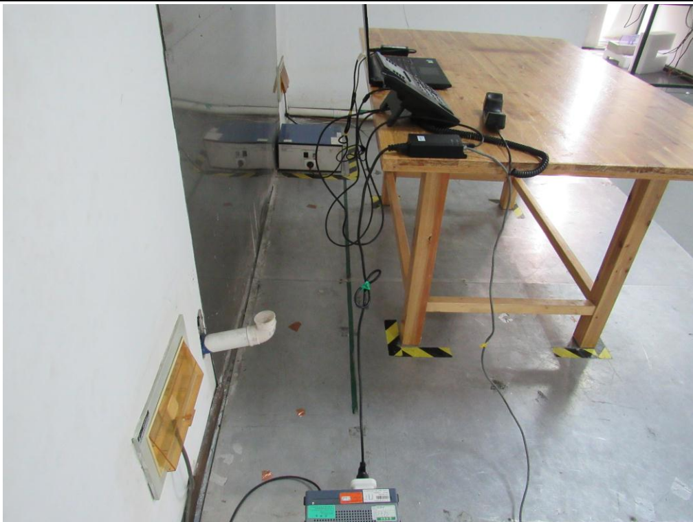
Conducted Emissions Test Setup Side View – POE
