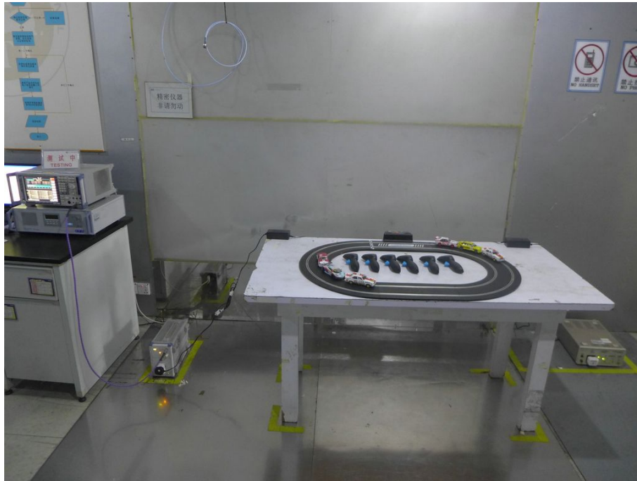
Conducted Emissions Test Setup
