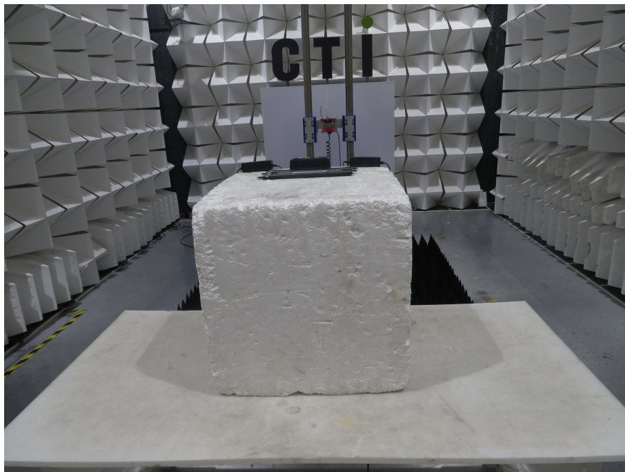
Radiated spurious emission Test Setup-2(Above 1GHz)
