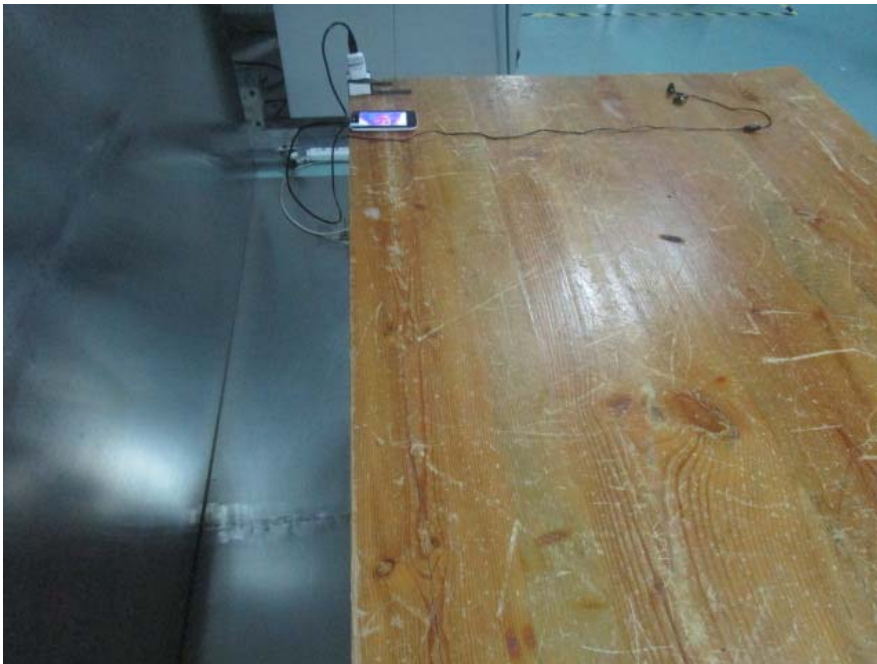
Conducted Emissions – Side View
