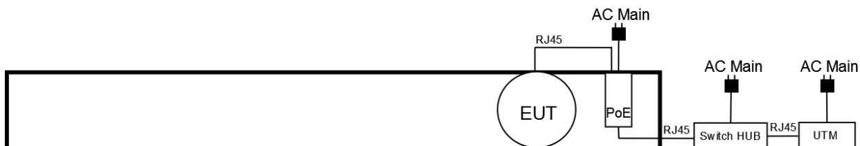
Test Setup Diagram - Radiated Emission Test
