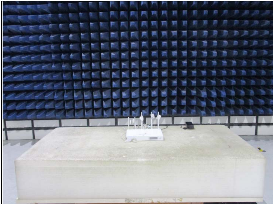
Radiated Emission Test below 1GHz
