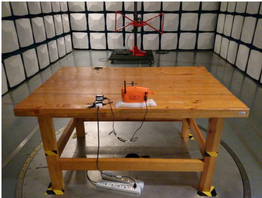
Radiated Emission –Rear View (Below 1GHz)
