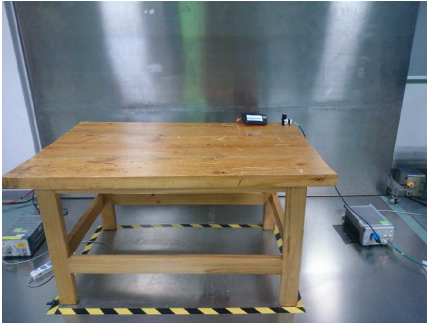
Conducted Emission--Front View
