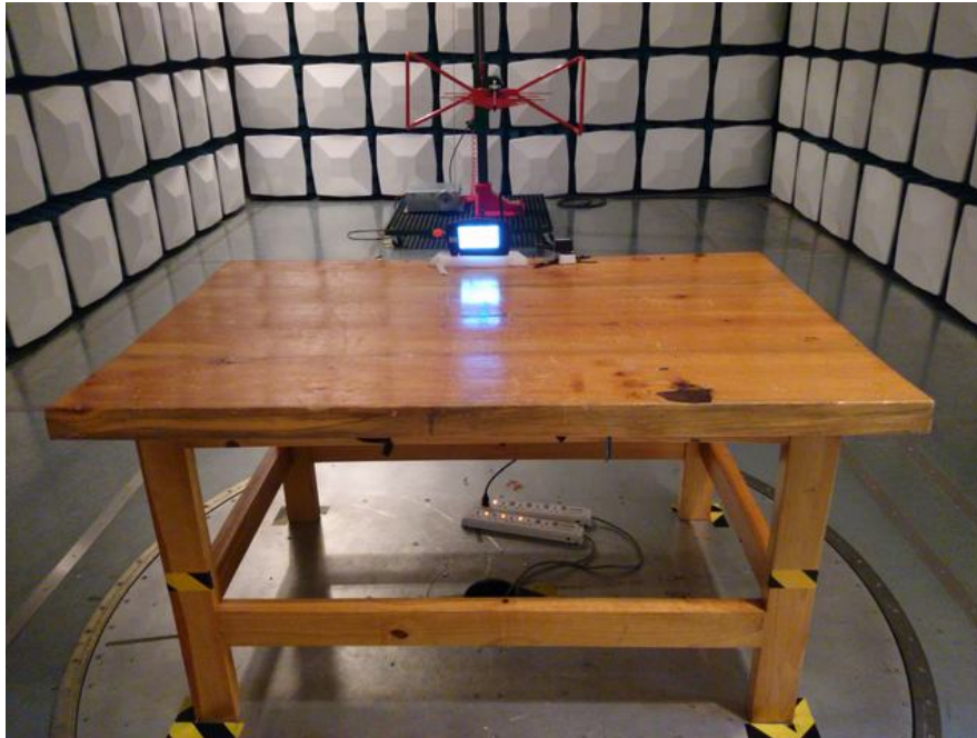
Radiated Emission –Front View (Below 1GHz)
