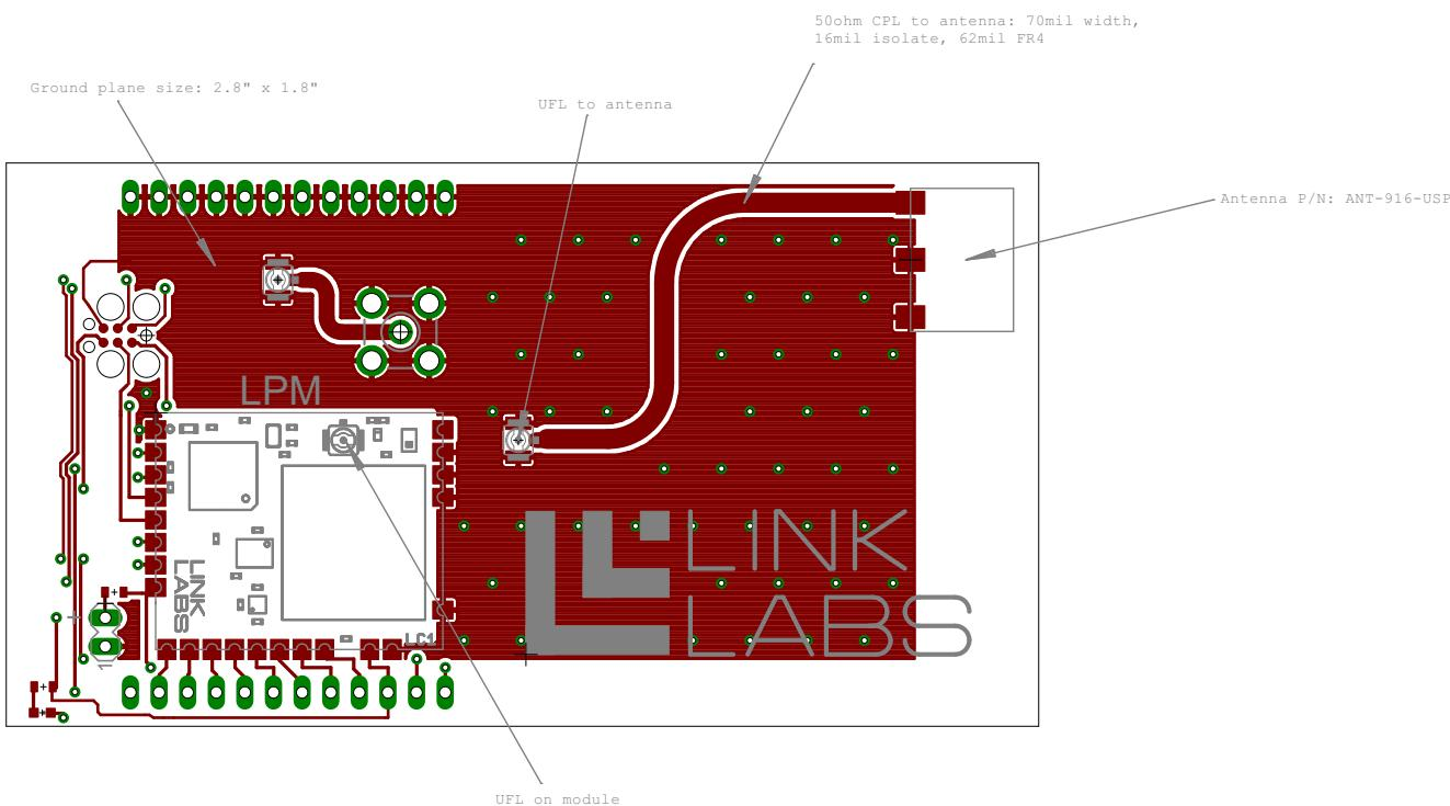
A reference layout design can be found in the Gerber file, *LL\_LP\_ChipAnt Reference.zip*.
