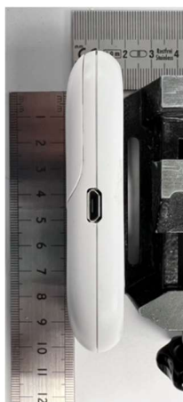
USB Port in Side of Meter
