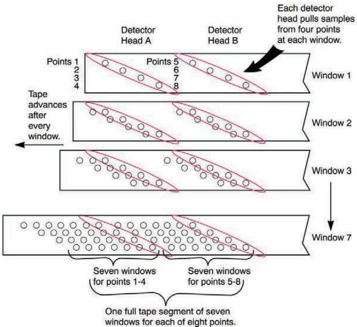
When monitoring a location, the system detects and measures a specific gas or a family of gases in the sample. The microprocessor in the analyzer module interprets the data and responds appropriately.
