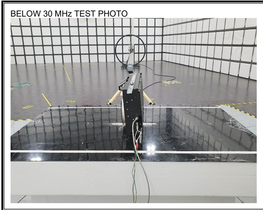
2) RADIATED RF MEASUREMENT SETUP (BELOW 1 GHz)
