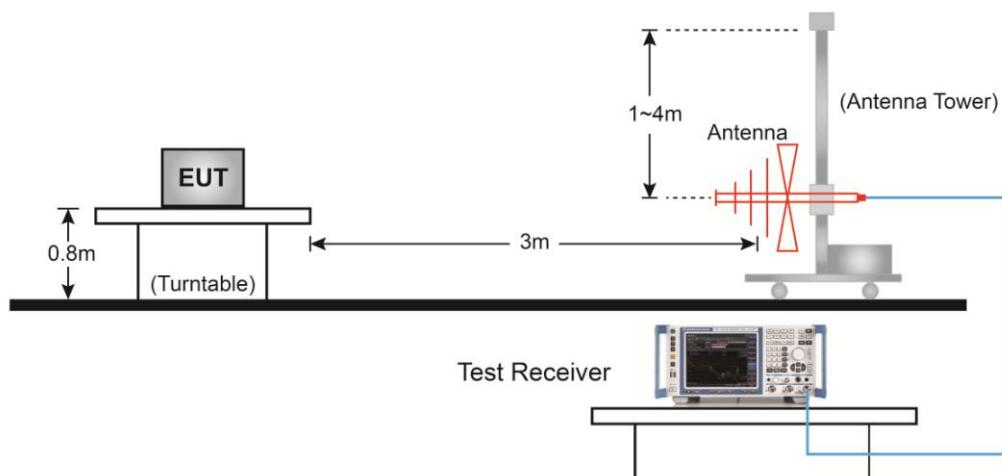
1GHz ~ 40GHz Test Setup:
