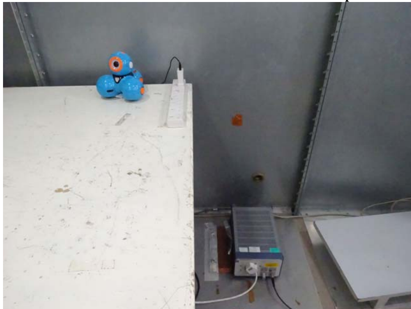
Measurement of Conducted Emission Test Set Up
