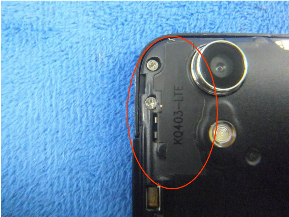
LTE - Antenna View
