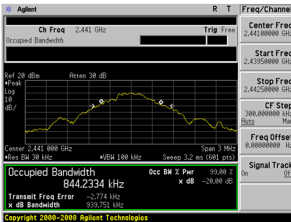
20dB Bandwidth plot on channel 78 (1Mbps)
