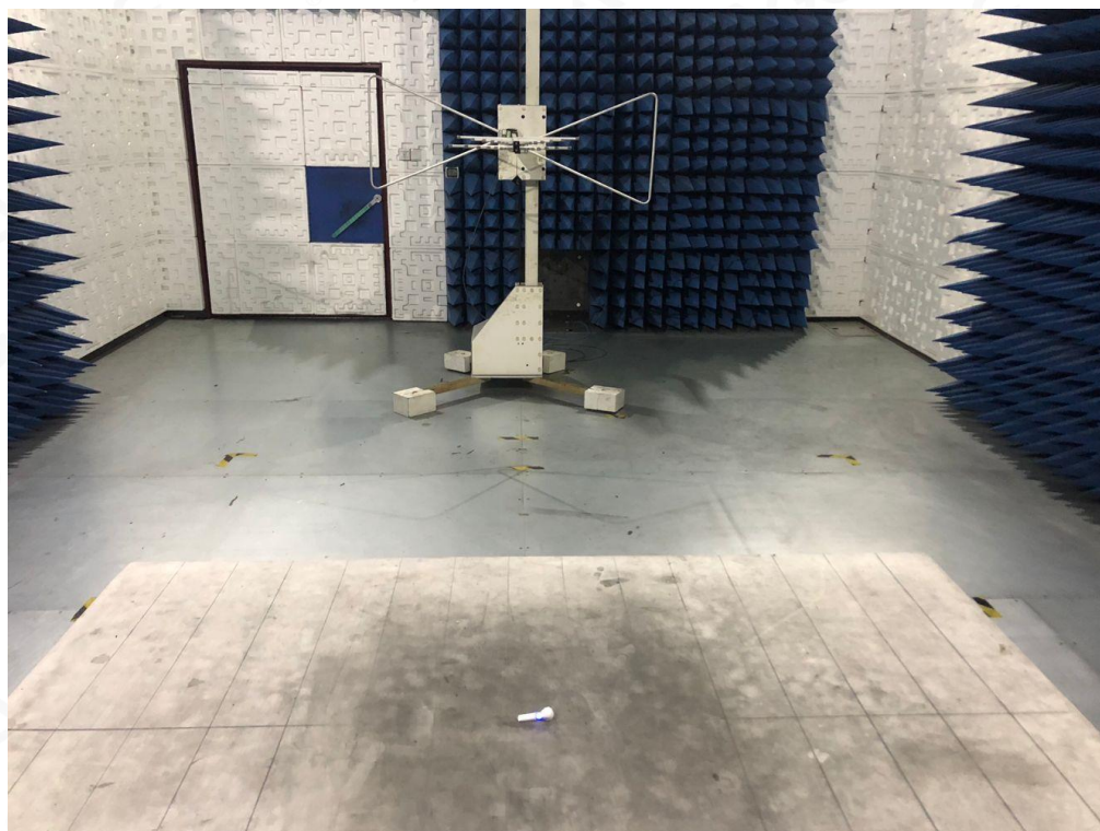
RADIATED EMISSION TEST SETUP ABOVE 1GHZ
