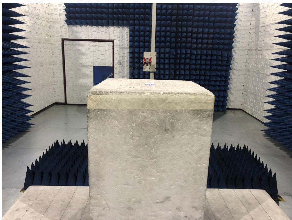
RADIATED EMISSION TEST SETUP ABOVE 1GHZ
