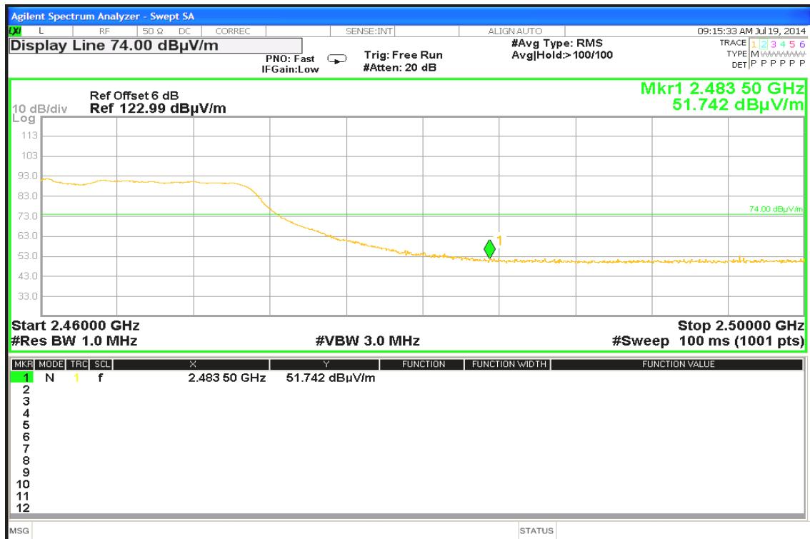
**Detector mode: Average****Polarity: Horizontal**
