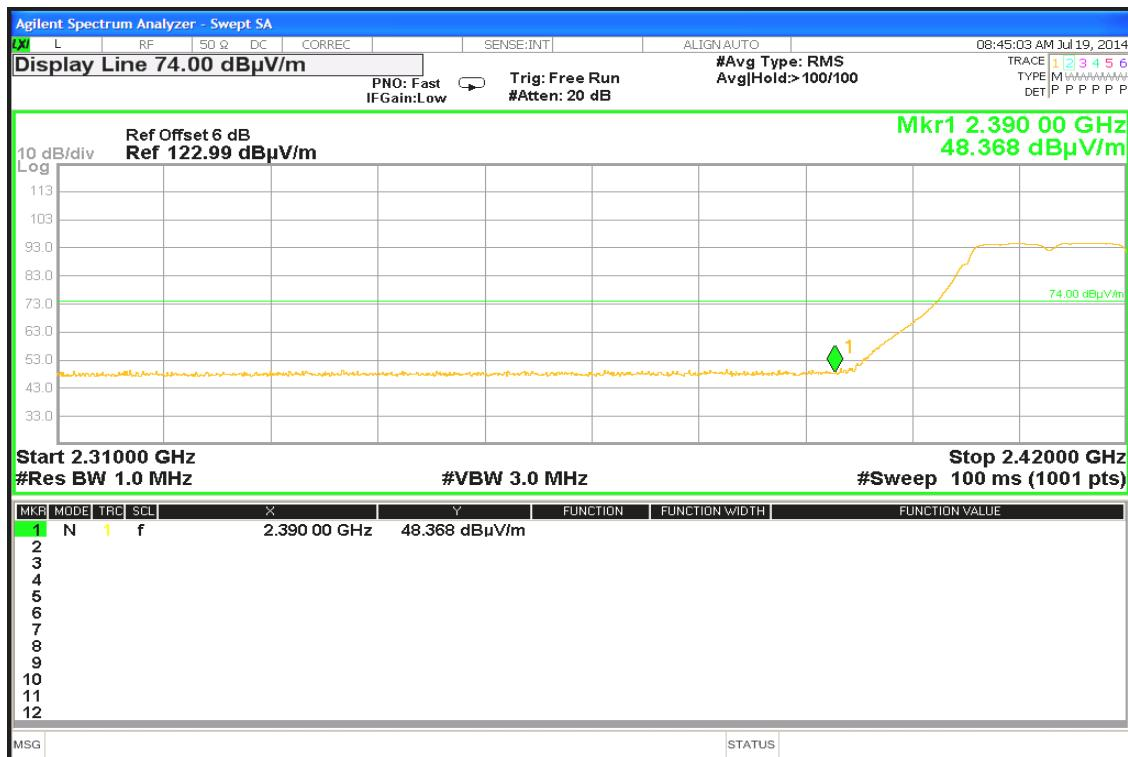
**Detector mode: Average****Polarity: Vertical**
