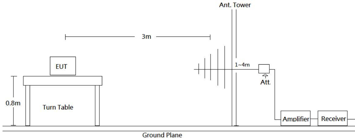
The radiated emission tests were performed in the 3 meters chamber test site, using the setup accordance with the ANSI C63.10-2013. The specification used was the FCC 15.209 and FCC 15.205 limits.
