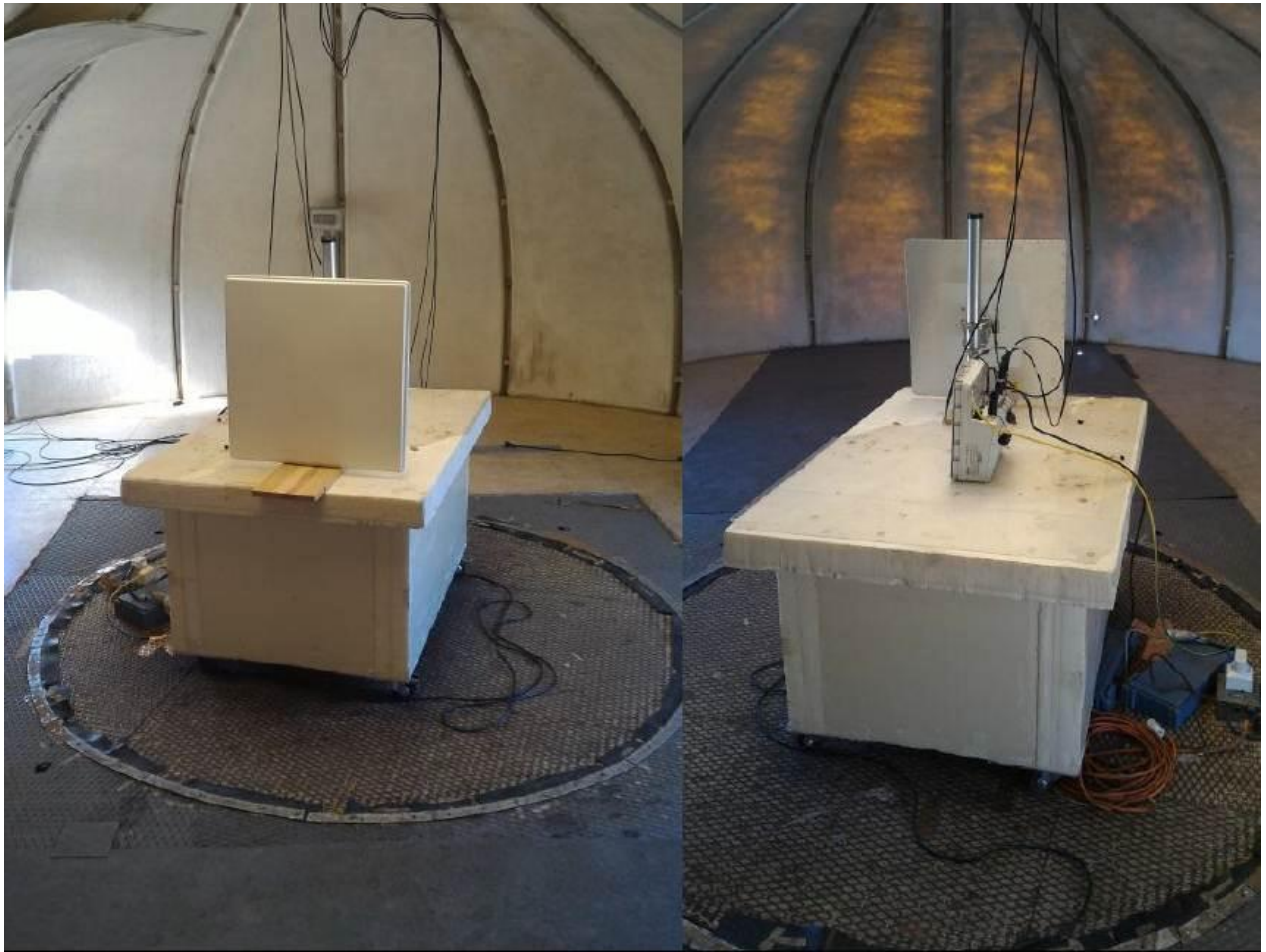
Test setup for radiated field strength (below 1GHz)
