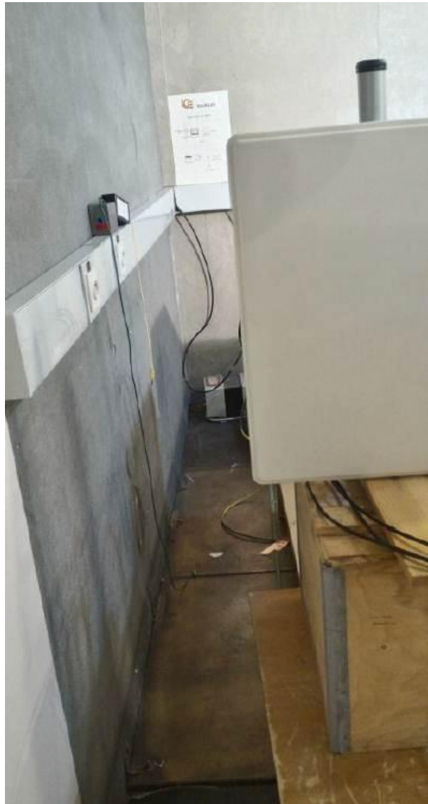
Test setup for power line conducted emissions
