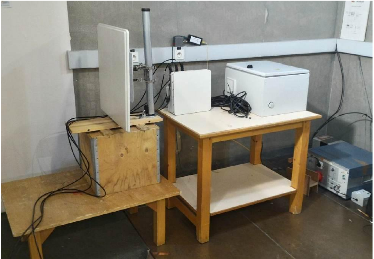
Test setup for power line conducted emissions
