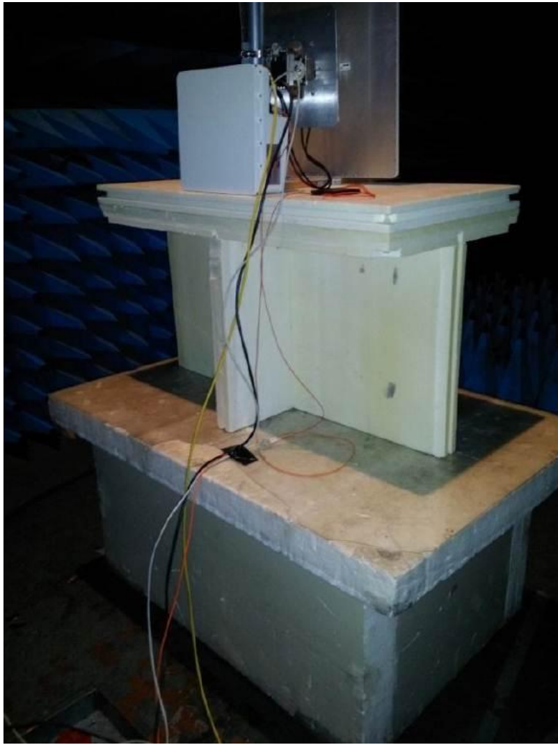
Test setup for radiated field strength (above 1GHz)
