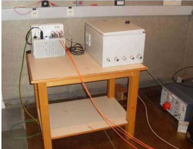
Test setup for power line conducted emissions
