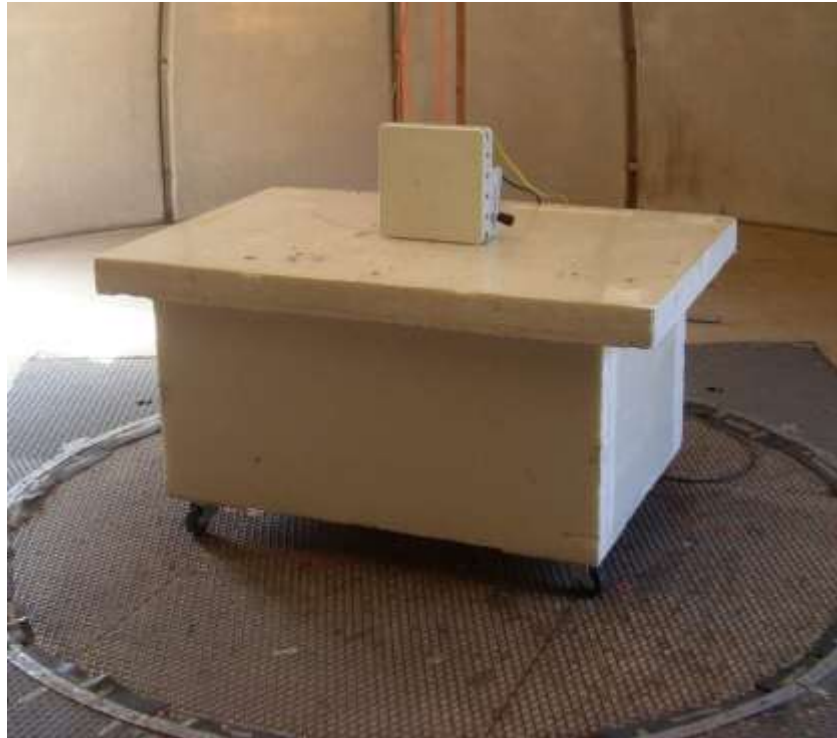
Test setup for radiated field strength
