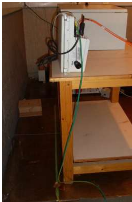
Test setup for power line conducted emissions
