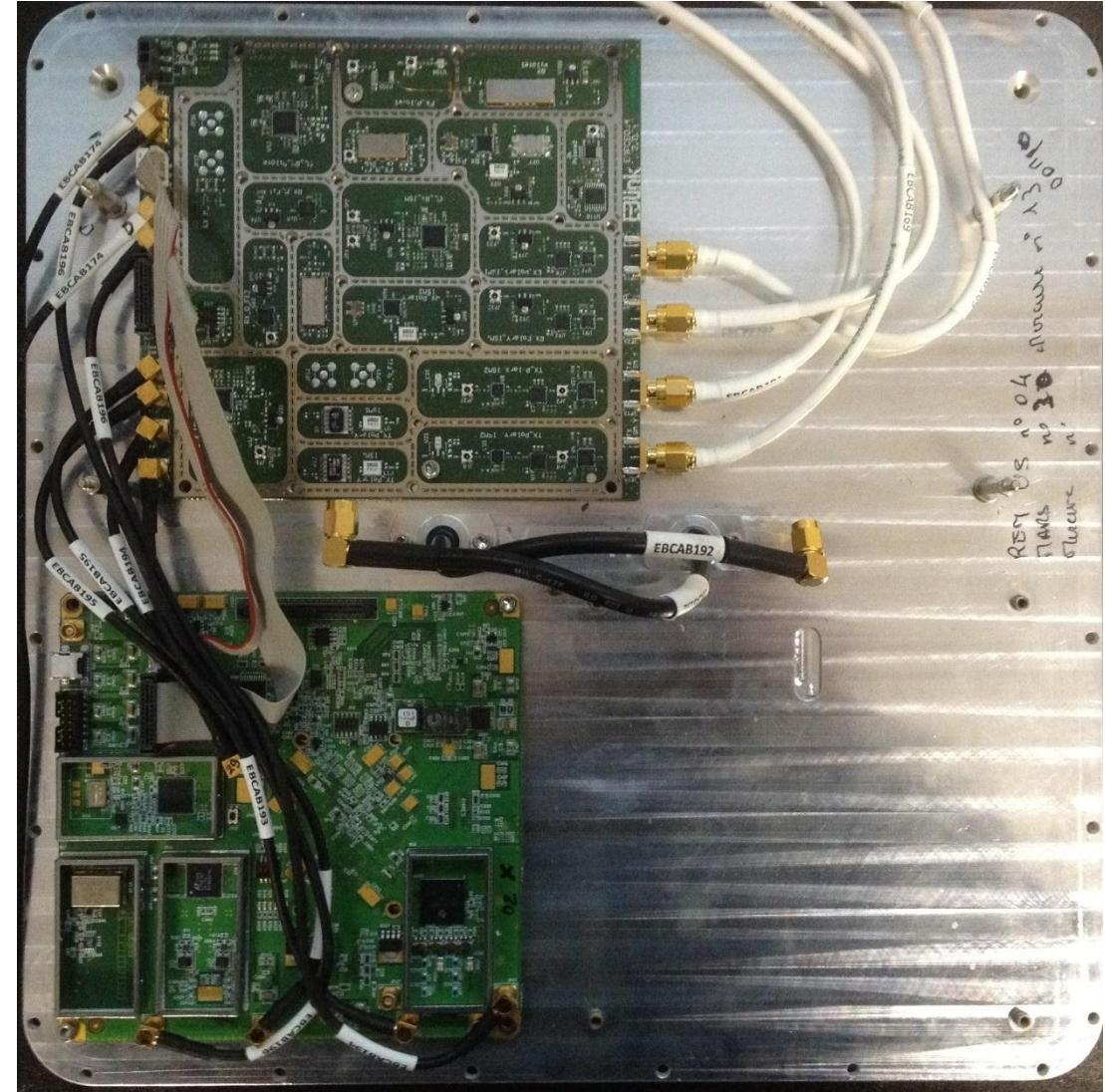
Antenna Radiator – EBBOARD61 and EBBOARD62/63 with Duplexors
