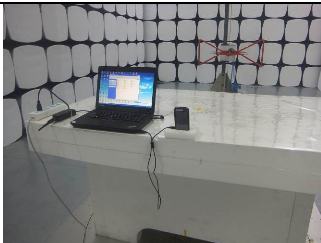
Radiated Spurious Emissions Test Setup Below 1GHz
