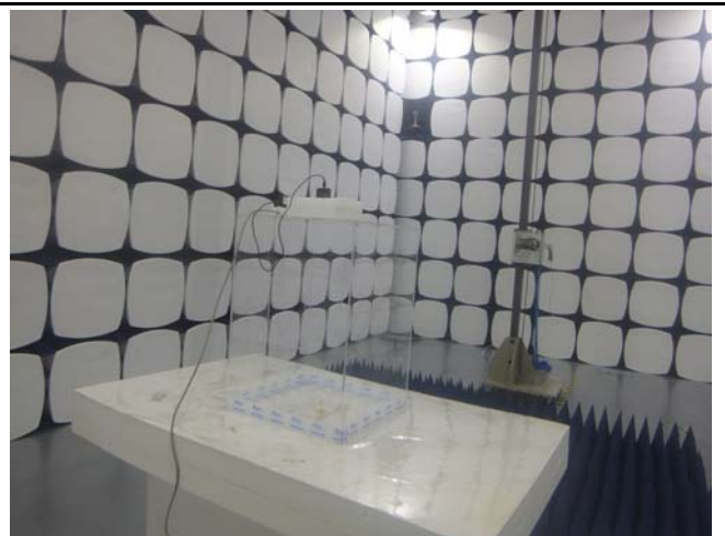
Radiated Spurious Emissions Test Setup Above 1GHz
