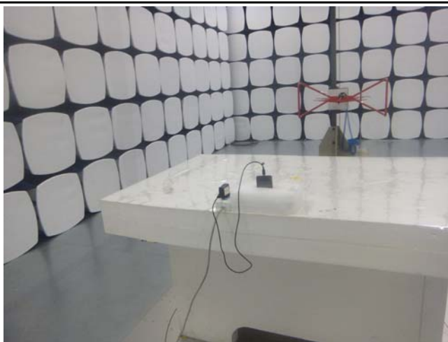
Conducted Emissions Test Setup Front View
