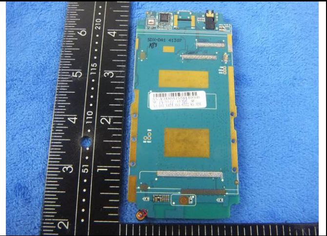
Mainboard Without Shielding - rear View
