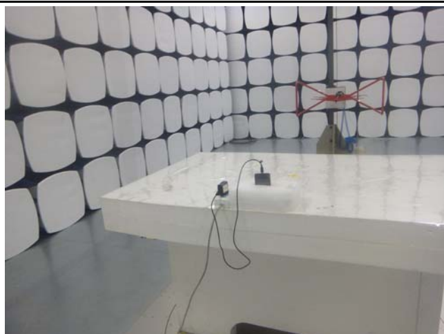
Conducted Emissions Test Setup Front View
