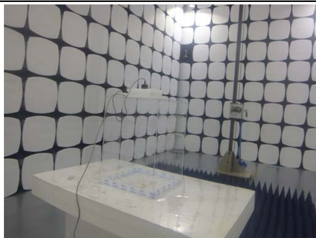
Radiated Spurious Emissions Test Setup Above 1GHz
