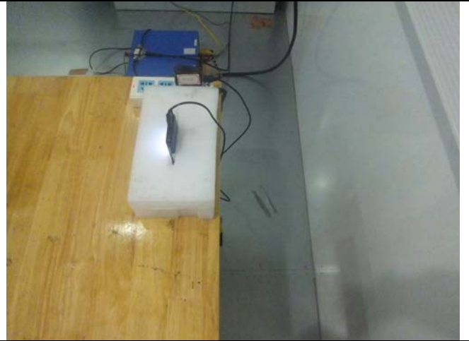
Conducted Emissions Test Setup Side View
