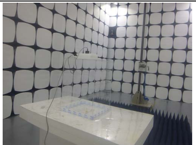
Radiated Spurious Emissions Test Setup Above 1GHz
