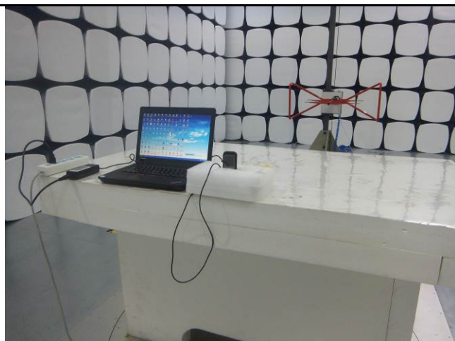
Conducted Emissions Test Setup – Front View
