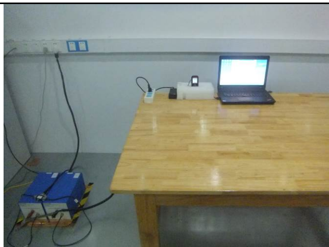
Conducted Emissions Test Setup – Front View
