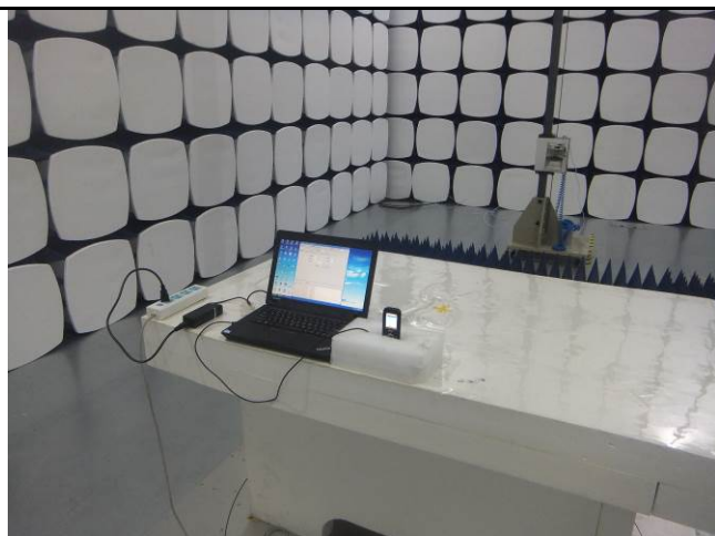
Radiated Spurious Emissions Test Setup Above 1GHz
