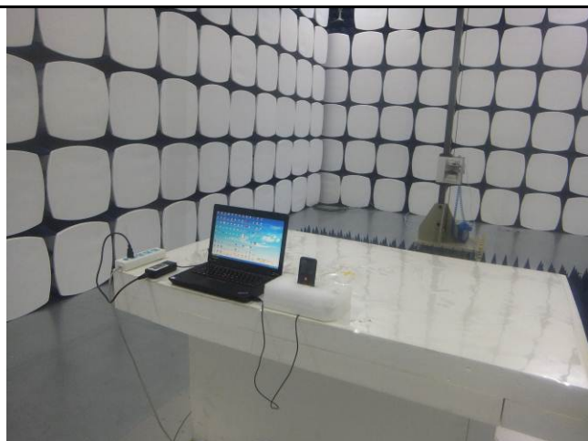
Radiated Spurious Emissions Test Setup Above 1GHz
