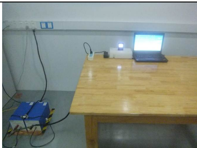
Conducted Emissions Test Setup – Front View
