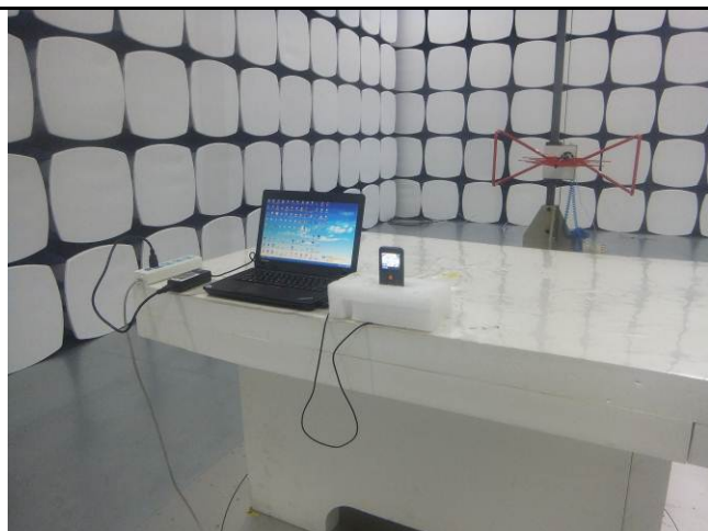
Conducted Emissions Test Setup – Front View
