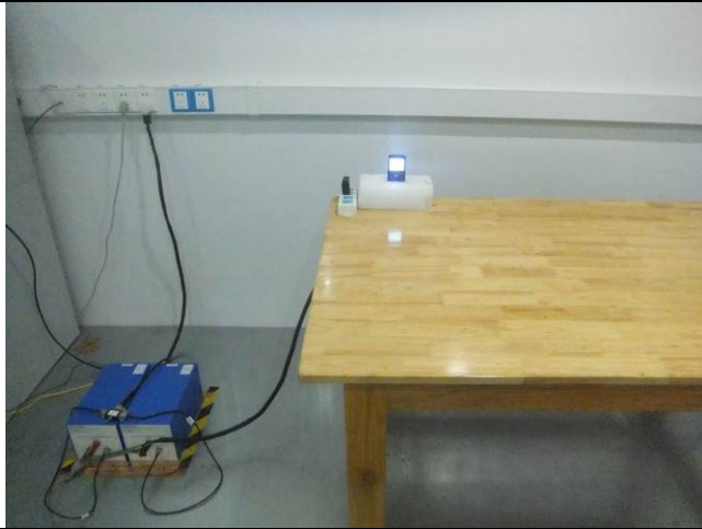
Conducted Emissions Test Setup Front View
