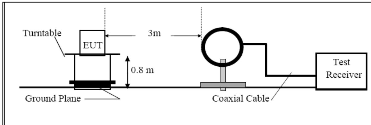
For Radiated Emission 30~1000MHz
