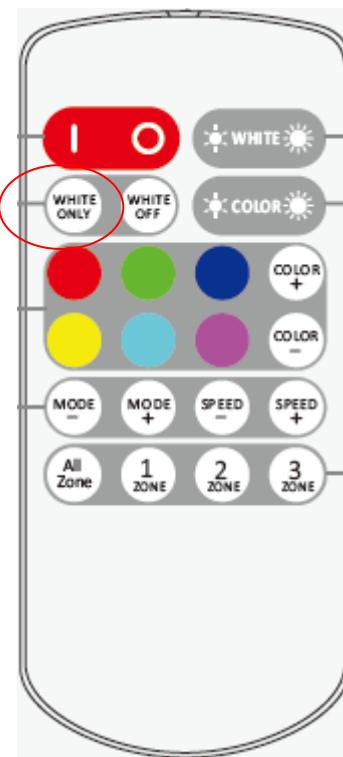
Note: All 24 buttons had been pre-tested and the worst case is the "WHITE ONLY" button. Also, only measurement data of worst case is recorded in the test report.
