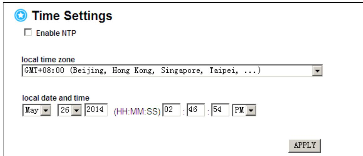
In the Time Settings interface, user can choose “Enable NTP” to make the device synchronize with an NTP network time server in time. Or you can manually set the local time zone, local date and time.
