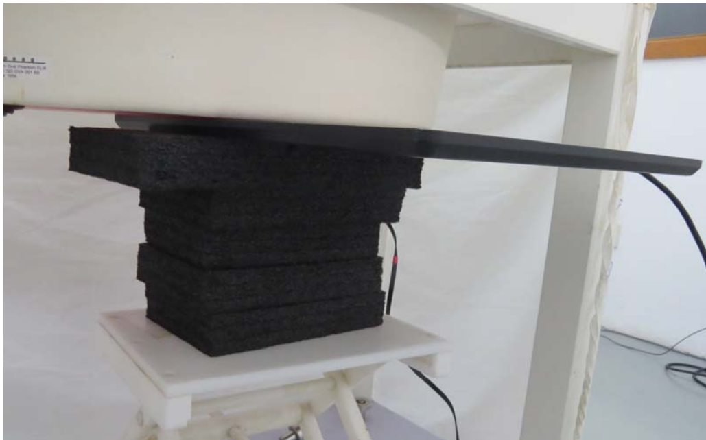
Picture 1: Front Side (Scan 1), the distance from EUT to the bottom of the Phantom is 0mm
