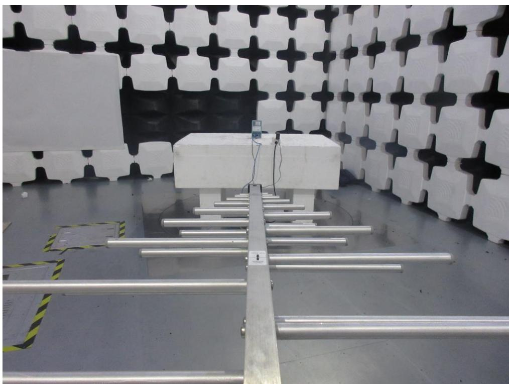
**Radiated Emissions Test Photos****Above 1 GHz**
