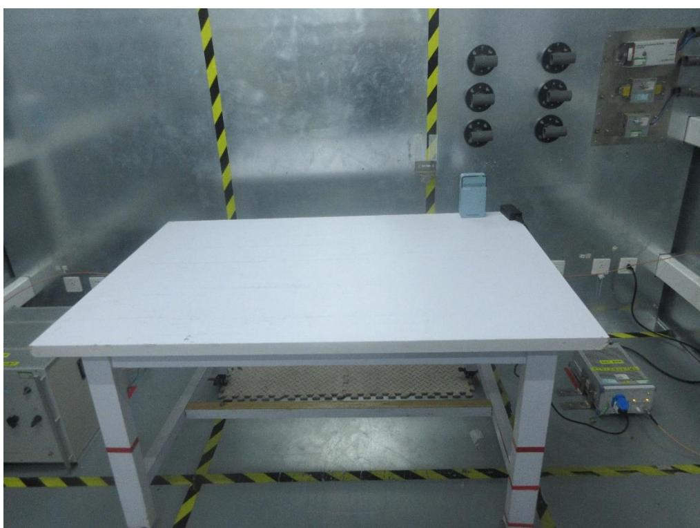
**Radiated Emissions Test Photos****30 MHz to 1000 MHz**
