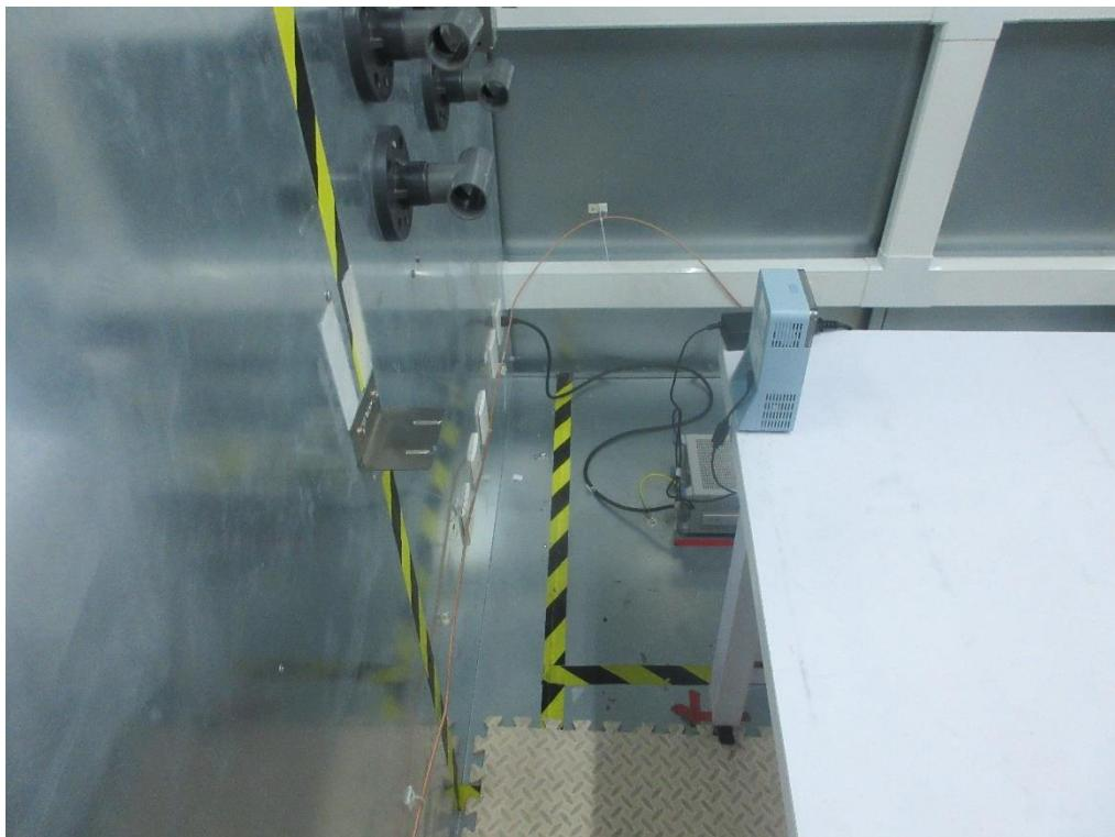
**Radiated Emissions Test Photos****30 MHz to 1 GHz**
