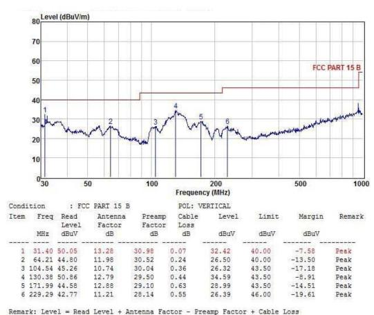
Remark: Level = Read Level + Antenna Factor - Freamp Factor + Cable Loss
