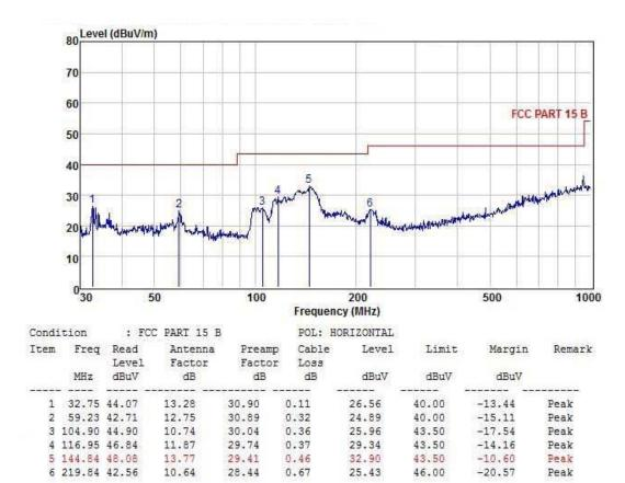
Remark: Level = Read Level + Antenna Factor - Preamp Factor + Cable Loss
