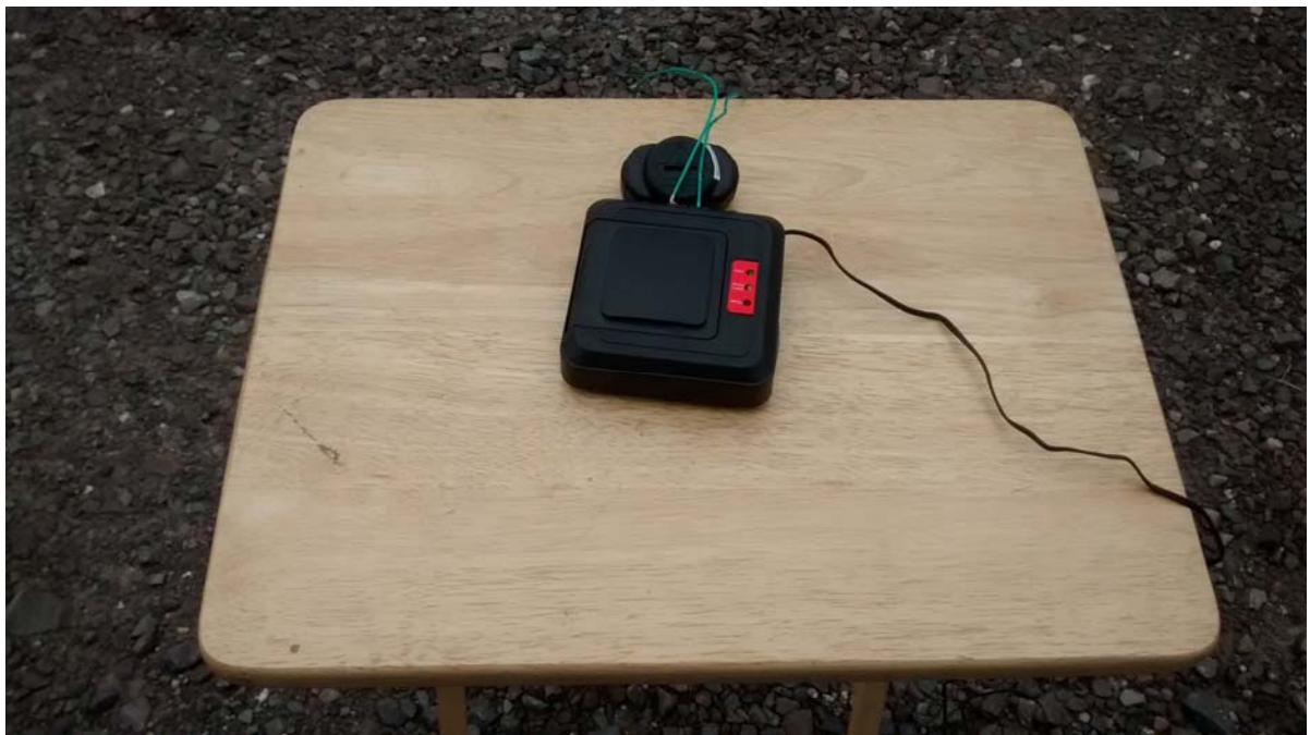
Figure 2: Radiated emissions setup 9 kHz to 30 MHz
