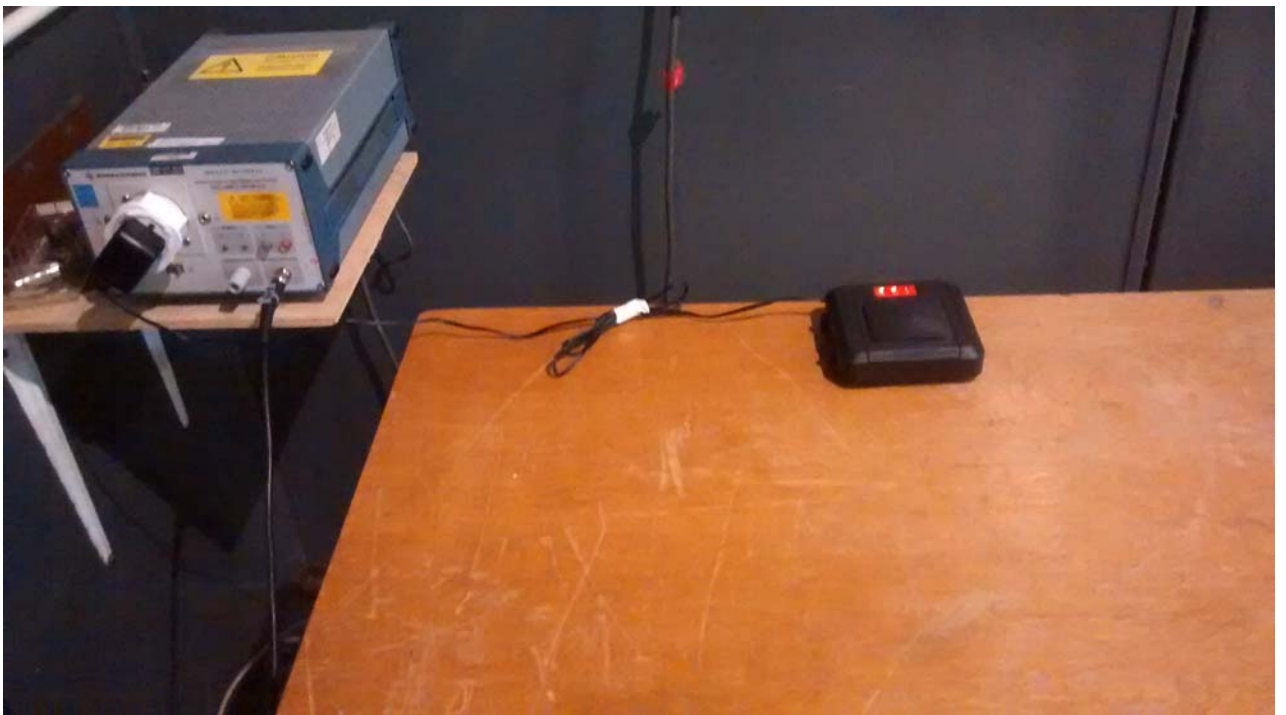
Figure 4: Conducted emissions setup
