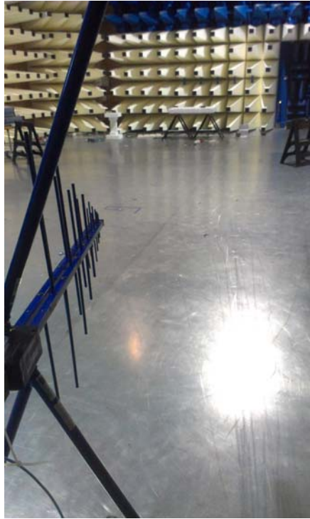
Figure 3: Radiated emissions anechoic chamber 30 MHz to 1 GHz
