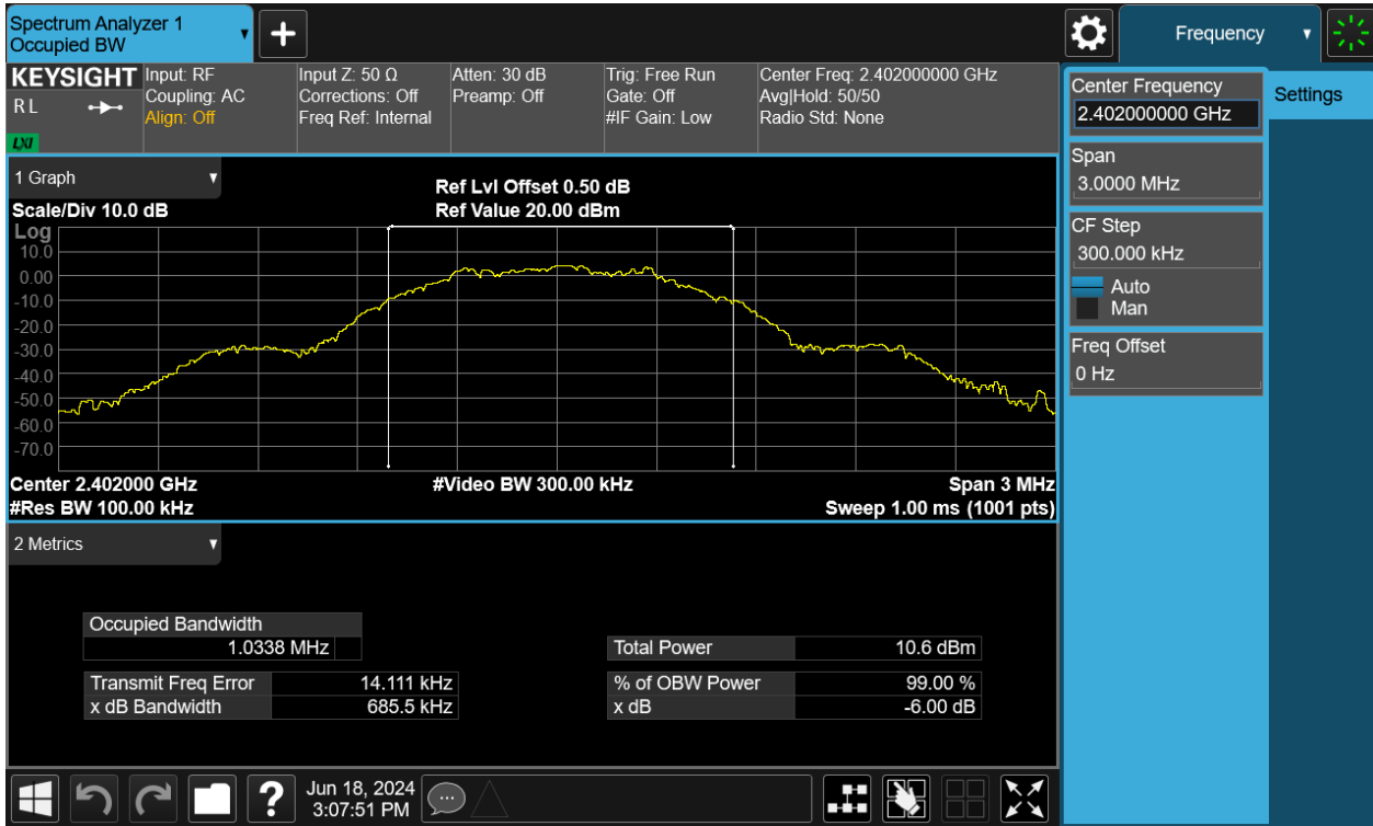
99% Bandwidth, 2402MHz, BLE-1Mbps
