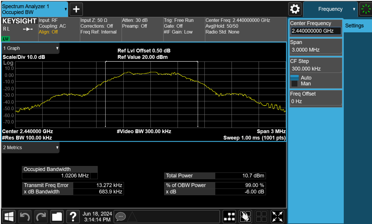
99% Bandwidth, 2440MHz, BLE-1Mbps
