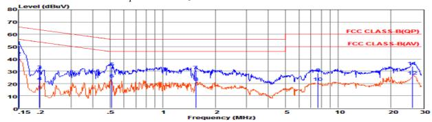
Env. Ins: EUT: M/N: Power Rating: Test Mode: Operator: 24\*/56% Tablet MAX STAR 6.0 AC 240V/60Hz TX-Low Channel(802.11b)
