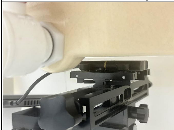
Horizontal-Up of EUT with 0.5 cm Gap
