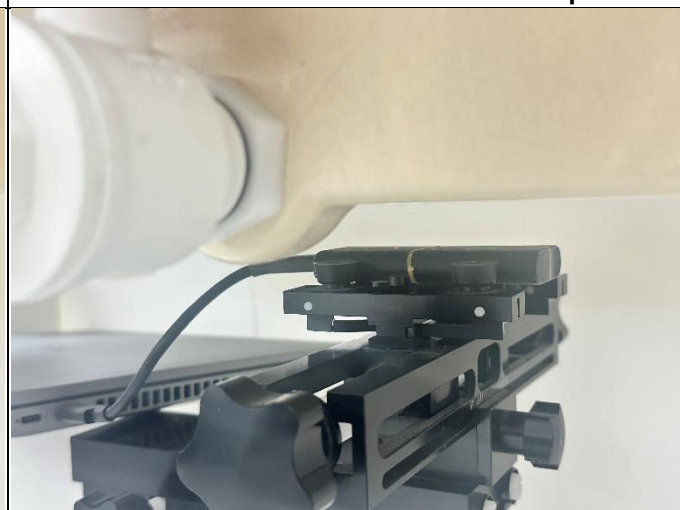
Horizontal-Down of EUT with 1.7 cm Gap
