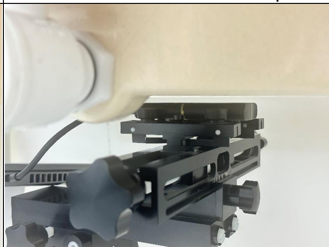
Horizontal-Down of EUT with 0.5 cm Gap
