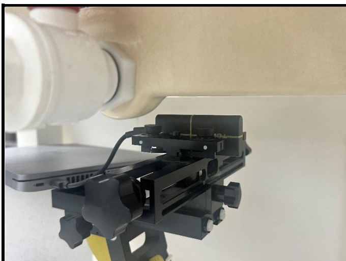
Vertical-Front of EUT with 1.7 cm Gap
