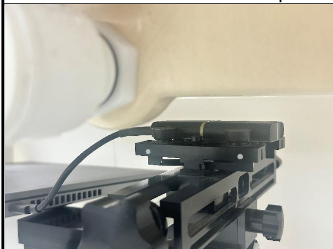
Horizontal-Up of EUT with 1.7 cm Gap
