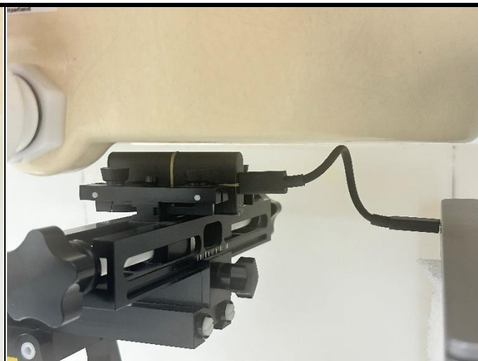
Vertical-Back of EUT with 0.5 cm Gap
