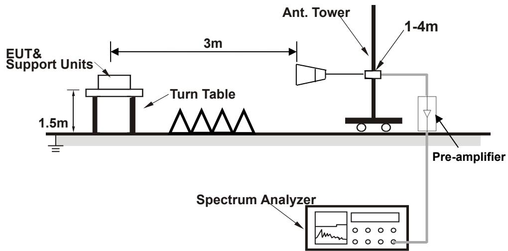
**For radiated test above 18GHz**
