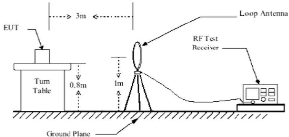
For radiated test from 30MHz to 1GHz
