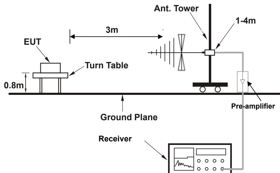
**For radiated test from 1GHz to 18GHz**
