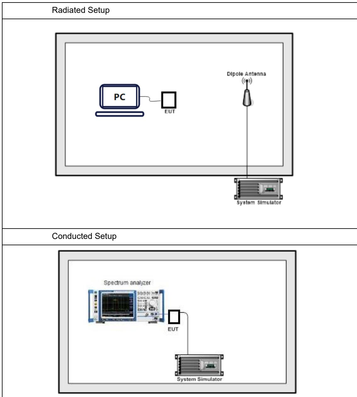
**Note:** This example is connection diagram of EUT test configurations. For detail, please refer to test mode configuration and setup photographs for each test item.
