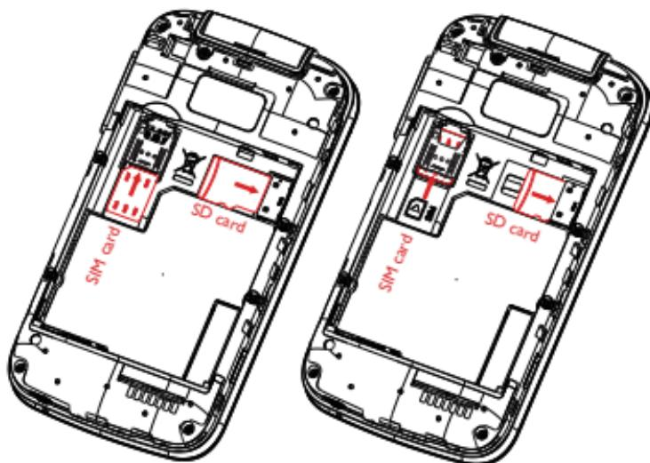
To remove the MicroSD card, press down on the small plastic tab holding the card in place, then slide out. Do not use force or any sharp objects.
