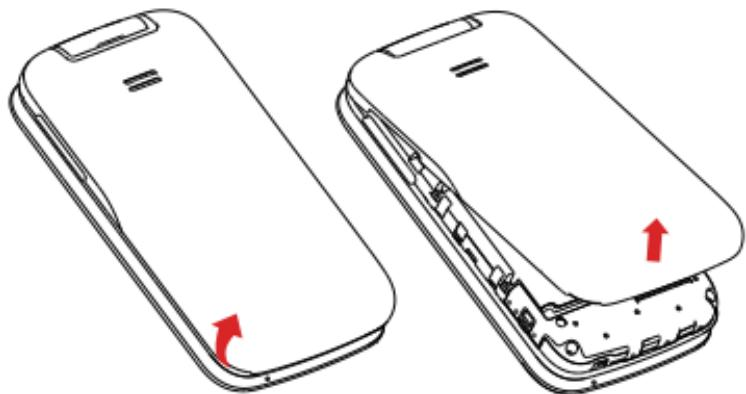
**Step 1.** With the device facing down, remove the back cover from the bottom left corner. Use your fingernail to carefully lift the cover away from the device body.
