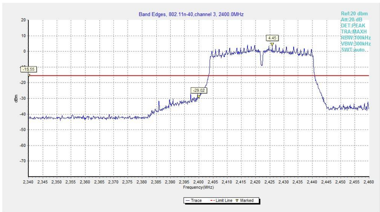
Fig.A.5.7 Band Edges (802.11n-HT40, Ch 3)
