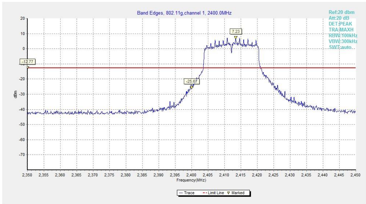
Fig.A.5.3 Band Edges (802.11g, Ch 1)
