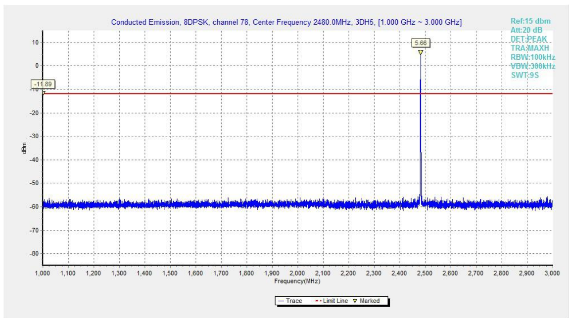
Fig.61. Conducted spurious emission: 8DPSK, Channel 78, 1GHz - 3GHz
