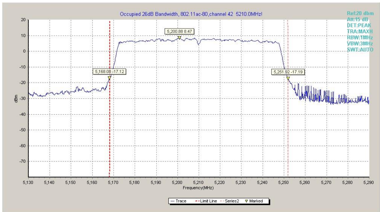
Fig.47 Occupied 26dB Bandwidth (802. 11ac-HT80, 5210MHz)
