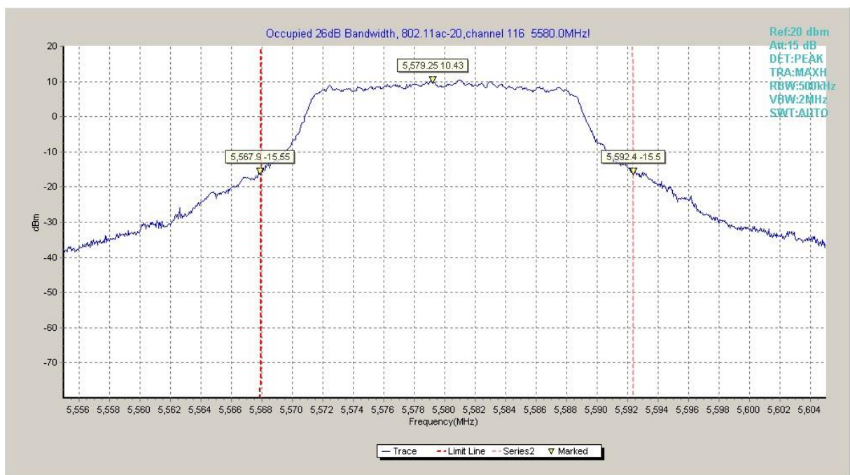
Fig.28 Occupied 26dB Bandwidth (802. 11ac-HT20, 5580MHz)
