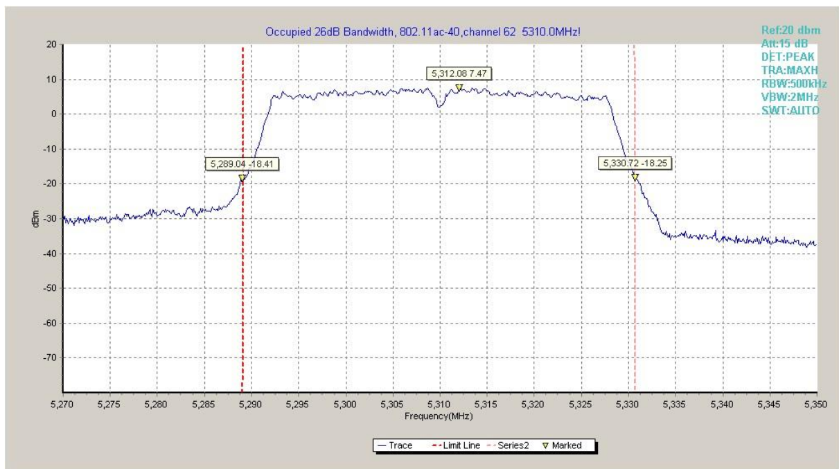
Fig.42 Occupied 26dB Bandwidth (802.11ac-HT40, 5310MHz)
