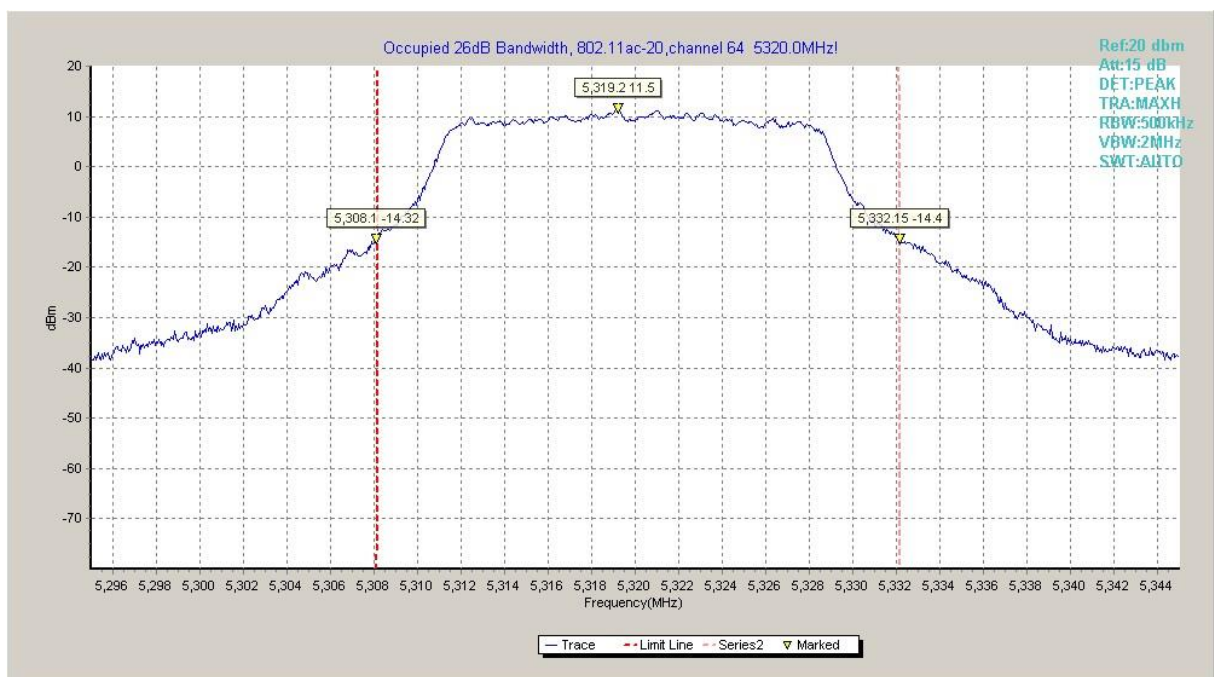
Fig.26 Occupied 26dB Bandwidth (802.11ac-HT20, 5320MHz)
