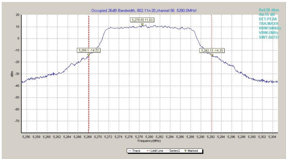
Fig.15 Occupied 26dB Bandwidth (802.11n-HT20, 5280MHz)
