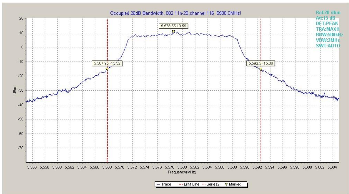
Fig.18 Occupied 26dB Bandwidth (802. 11n-HT20, 5580MHz)
