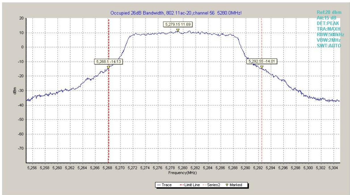
Fig.25 Occupied 26dB Bandwidth (802.11ac-HT20, 5280MHz)
