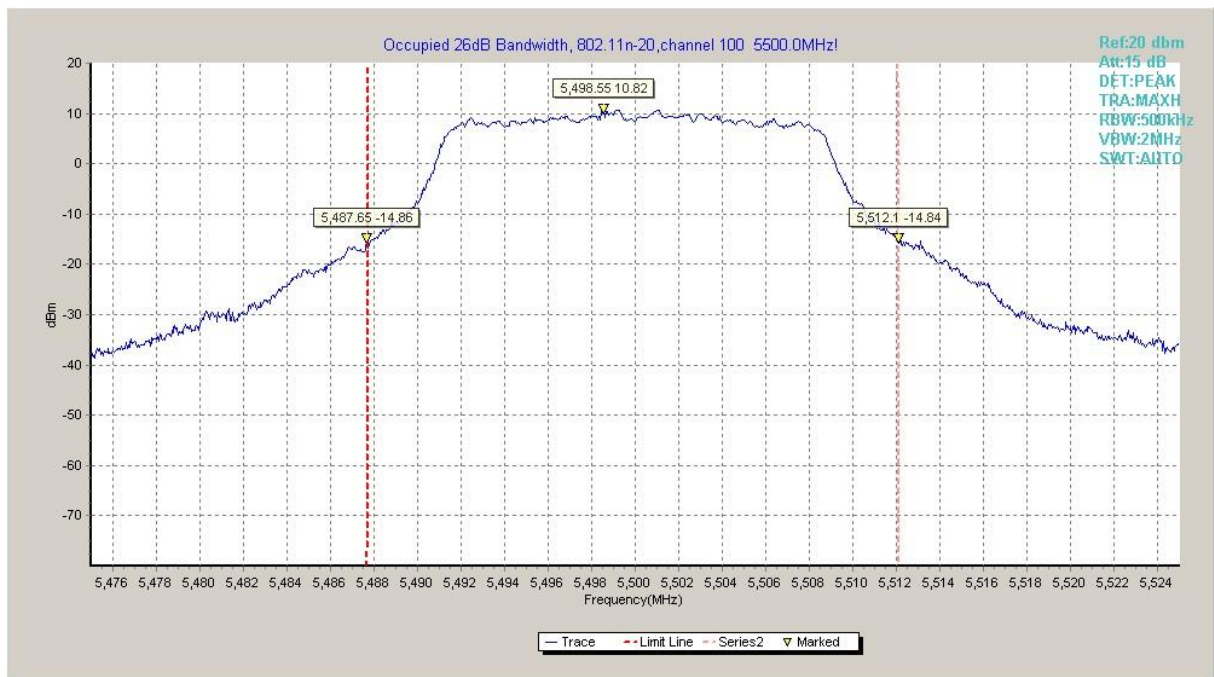
Fig.17 Occupied 26dB Bandwidth (802. 11n-HT20, 5500MHz)
