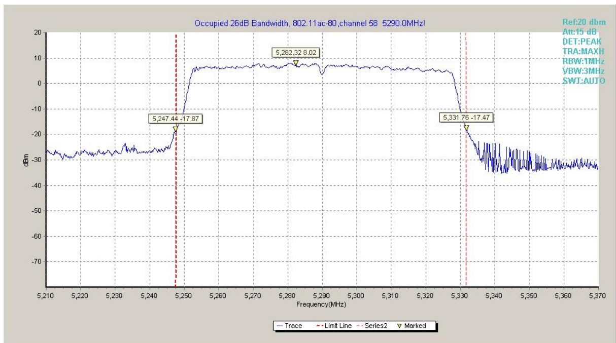
Fig.48 Occupied 26dB Bandwidth (802. 11ac-HT80, 5290MHz)
