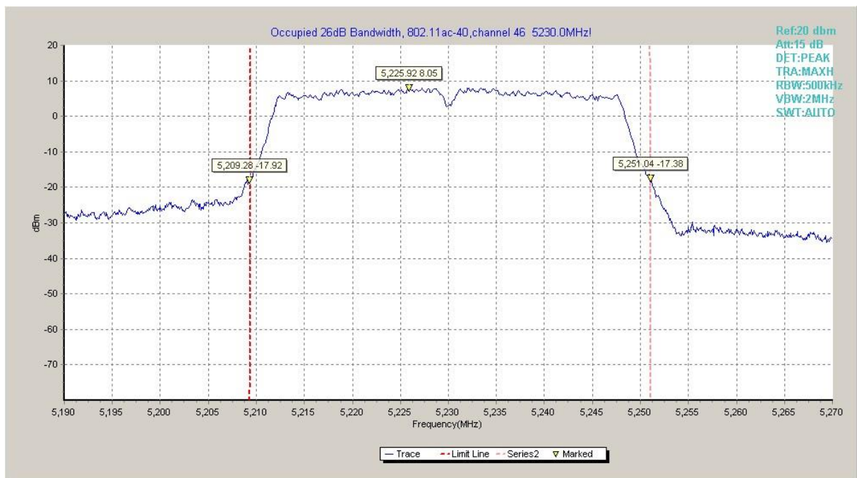
Fig.40 Occupied 26dB Bandwidth (802.11ac-HT40, 5230MHz)
