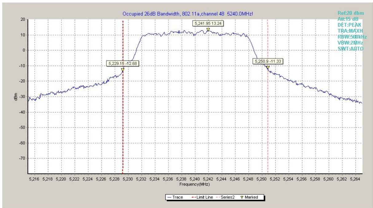
Fig.3 Occupied 26dB Bandwidth (802.11a, 5240MHz)
