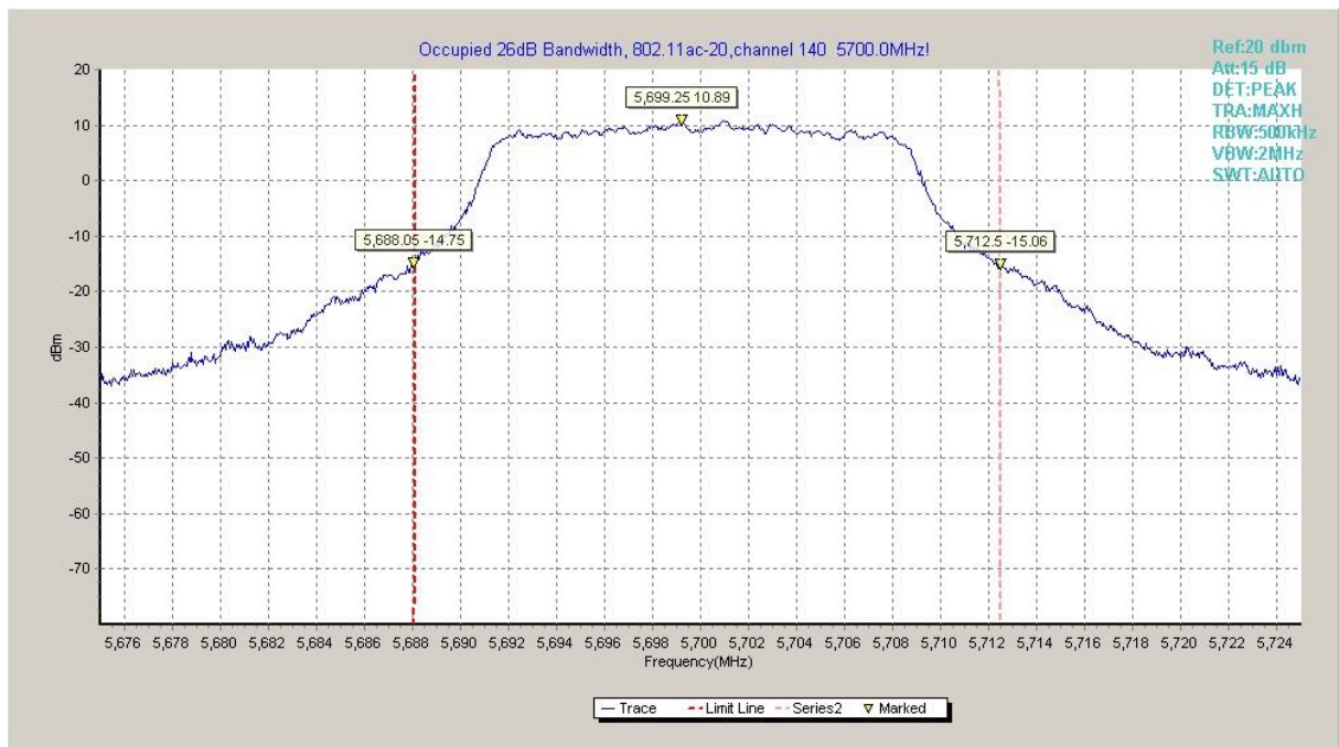
Fig.29 Occupied 26dB Bandwidth (802. 11ac-HT20, 5700MHz)
