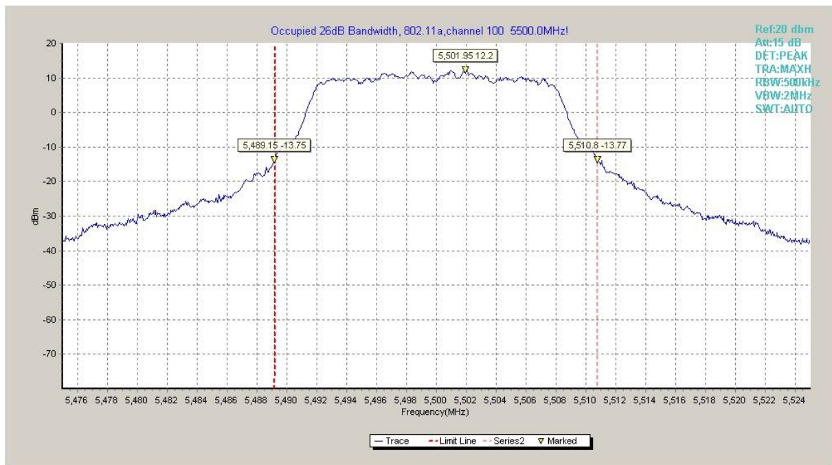
Fig.7 Occupied 26dB Bandwidth (802.11a, 5500MHz)
