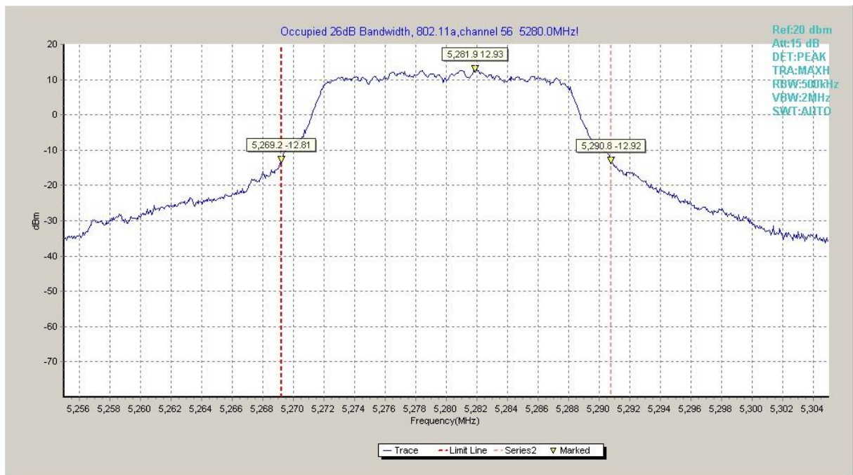
Fig.5 Occupied 26dB Bandwidth (802.11a, 5280MHz)
