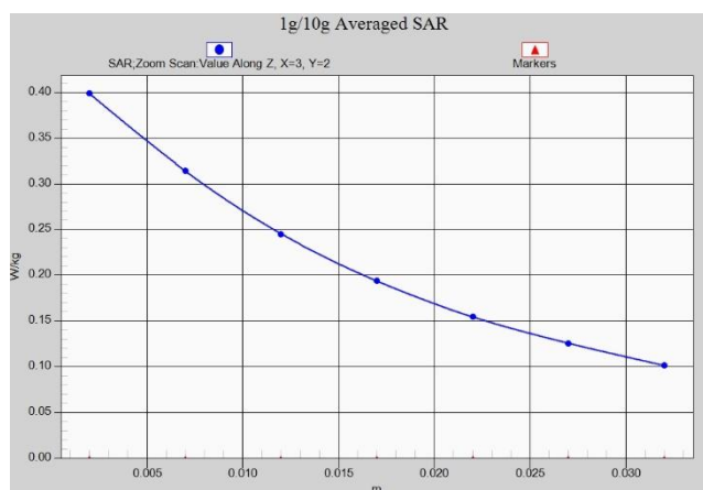
Fig. 1-1 Z-Scan at power reference point (GSM850)
